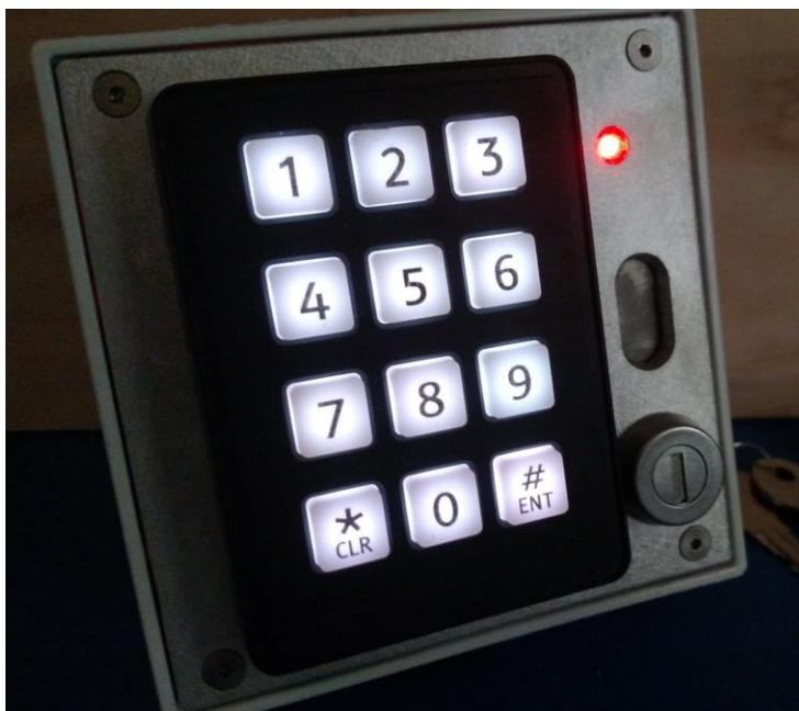
Up to 2000 user codes (up to 10 digits long) or cards can be easily programmed into the controller with the flash drive using the included software, which will automatically update user status by date and can import real-time changes to the user database from a third party user management program.
